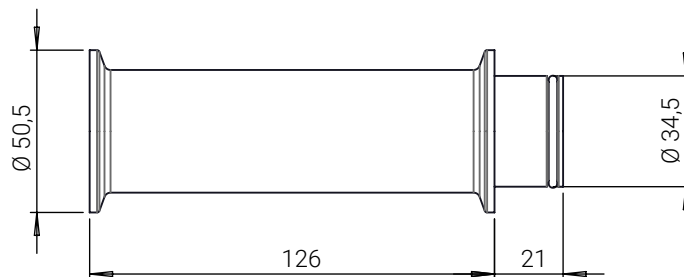
The overall diameter of the UKK is 50,5 mm. The distance between the tri-clamp connections is 126 mm.
